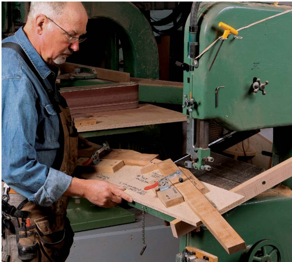
One jig, two legs, two angles. The angled table (18°) and jig combine to cut a compound angle on both legs in one shot. A wooden guide bar on the bottom rides in the table's miter slot.
