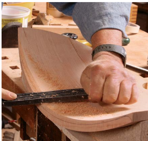
Soften the edges. Fortune hogs off most of the waste with a Shinto saw rasp and then follows up with files (left) and sandpaper. To smooth the curves, use a sanding block that's been shaped to match the radius (right). Wrap the sandpaper around the ends of the block and staple it in place.
