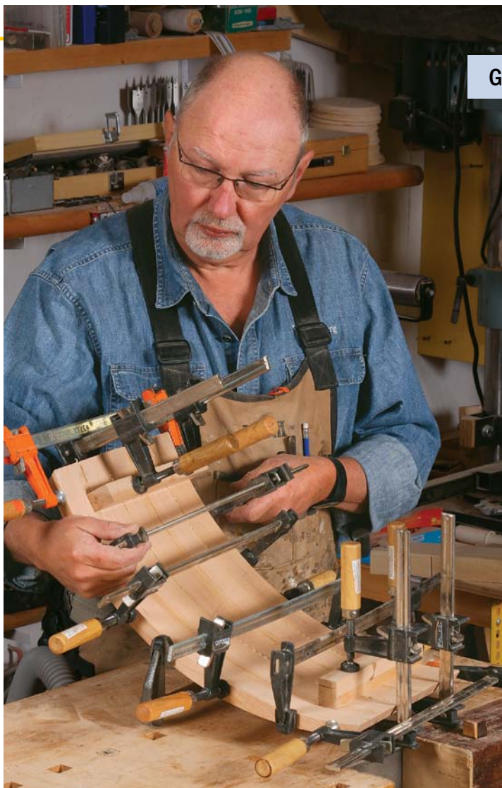
Clamp it up in sections. Fortune starts by gluing up pairs of ribs and then glues those together into a single blank. Cauls across the blank's width keep the ribs aligned, which makes it much easier to smooth it.
