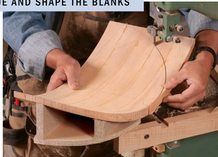
Cut it out at the bandsaw. Use hot-melt glue to hold the blank in place. Fortune puts the blank in the cradle first and then adds a few drops of glue along the seams.
