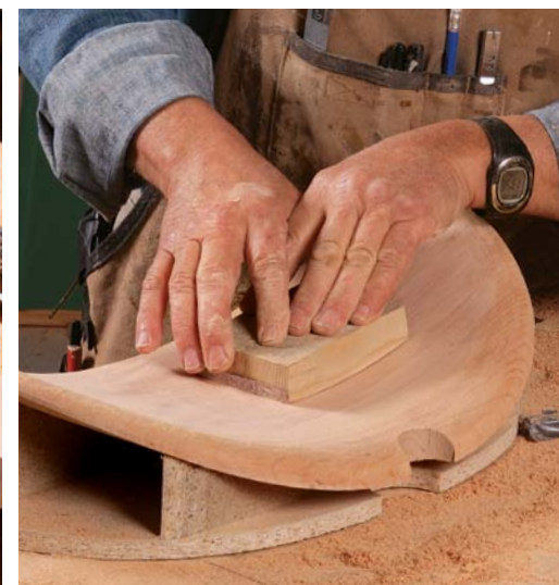
Soften the edges. Fortune hogs off most of the waste with a Shinto saw rasp and then follows up with files (left) and sandpaper. To smooth the curves, use a sanding block that's been shaped to match the radius (right). Wrap the sandpaper around the ends of the block and staple it in place.
