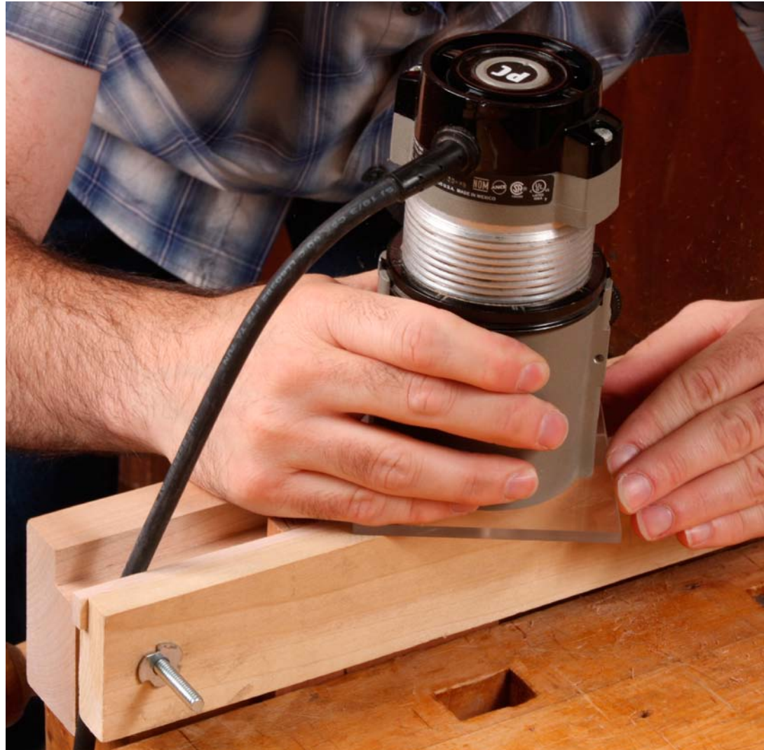
Rout away. This can be scary, because a router can really mess things up quick. Practice, a steady hand, and a healthy dose of confidence (or a devil-may-care attitude) is all you need to control the router.
