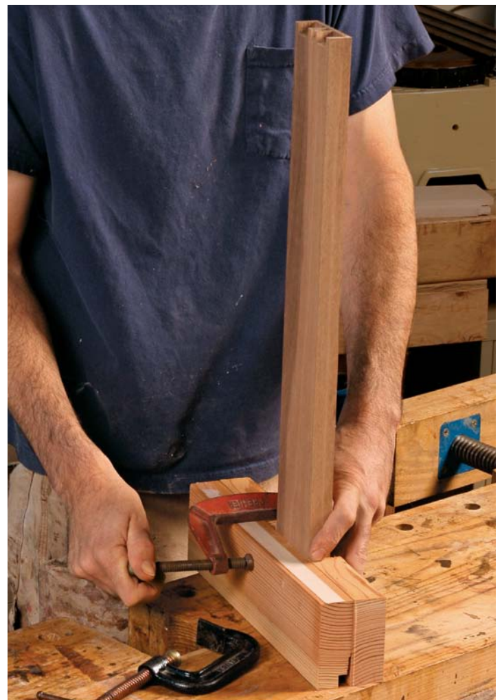
Router jig is easy to set up. Use your benchtop to bring the top of the jig level with the drawer front. Then clamp it in place.
