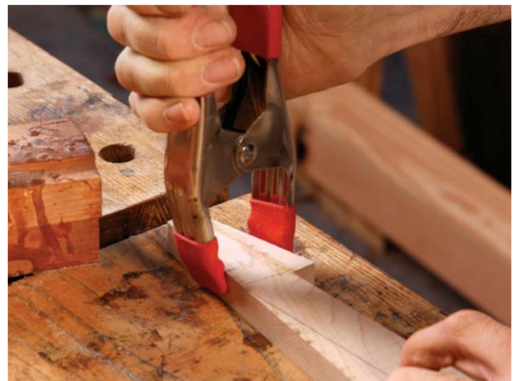
Glue on a stop. Put it at the narrow end, which leads into the blade, so that the jig can handle drawer sides of any length.
