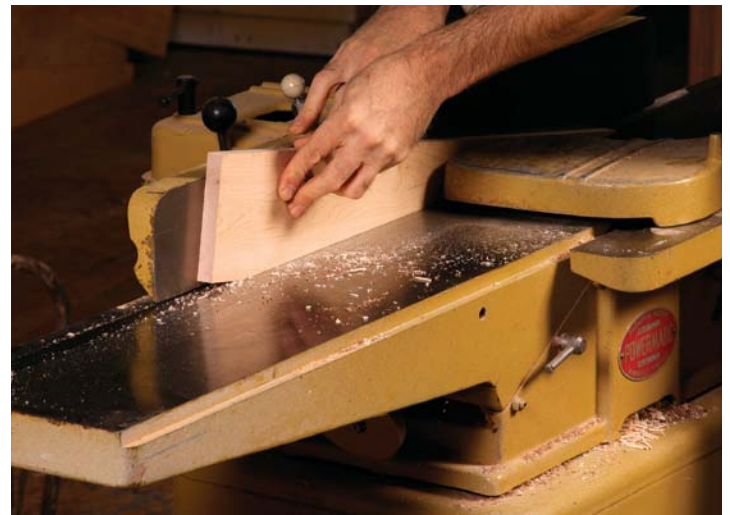
Joint the taper for a clean edge. It's fast and accurate. You also could use a handplane.
