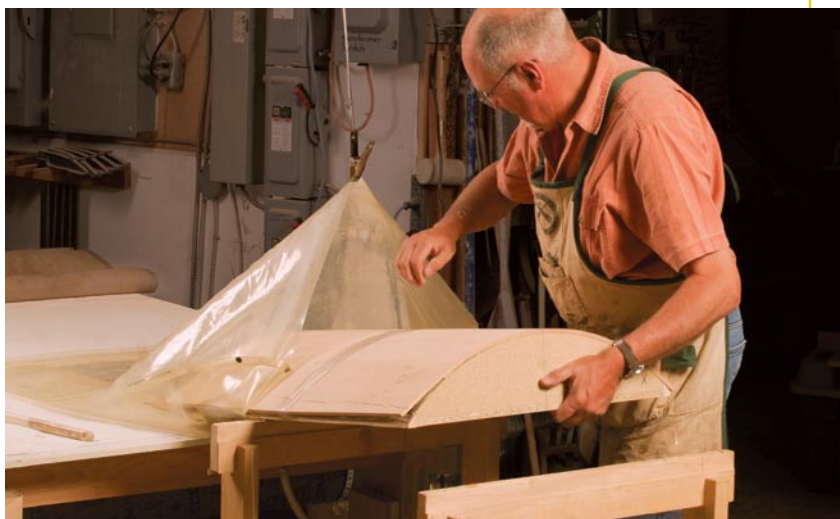
In the bag. The press applies uniform pressure from all directions, so there won't be any bumps in the form. Leave it in the bag overnight.
