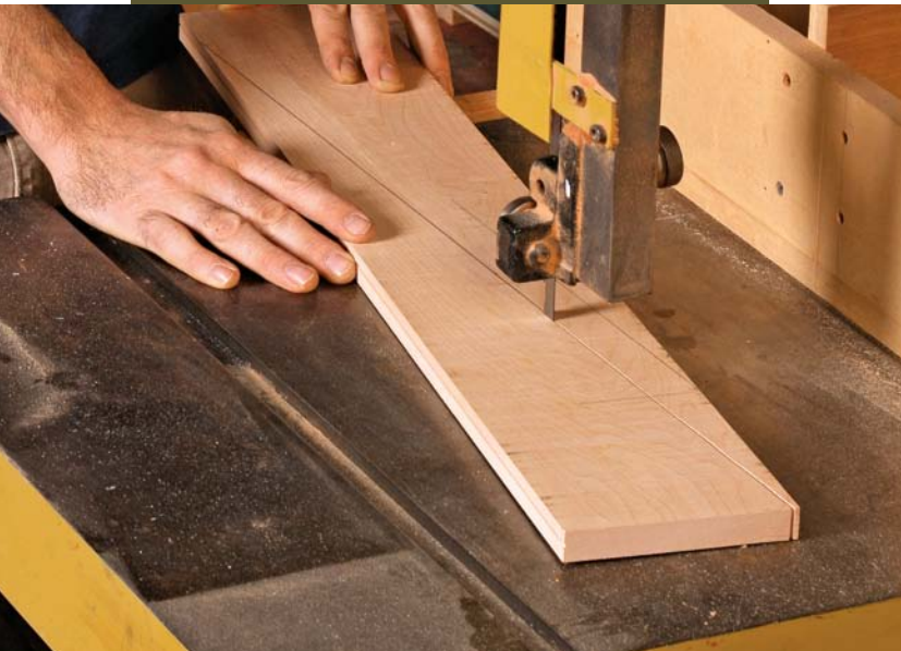
Taper the jig to match the tails. It should be several inches longer than the drawer sides.
