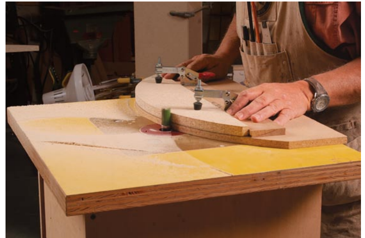
Pattern jig creates matching ribs. Fortune cuts his pattern oversize, then adds a fence and some toggle clamps to make routing the ribs quick, safe, and accurate.
