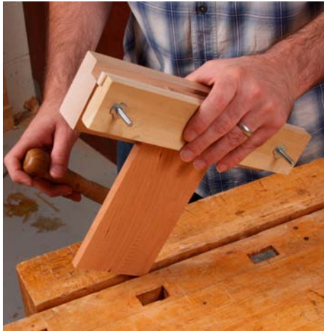
The whole contraption goes in your vise. But only the pin board is clamped. The jig rests on top of the vise jaw and bench.
