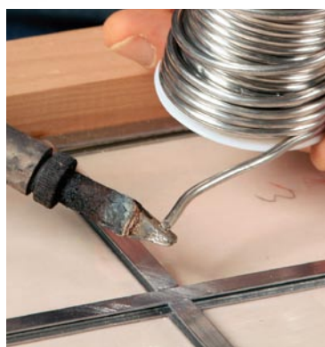
Solder on. Melt some solder onto the iron (left), and apply it to the joint (right). Do not leave the iron in contact with the came too long or it will melt the came and create a gap.
