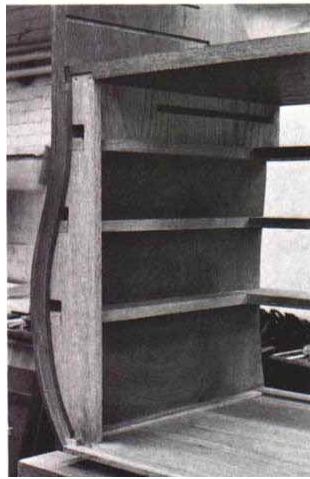
Notched vertical members support drawer runners at back.
