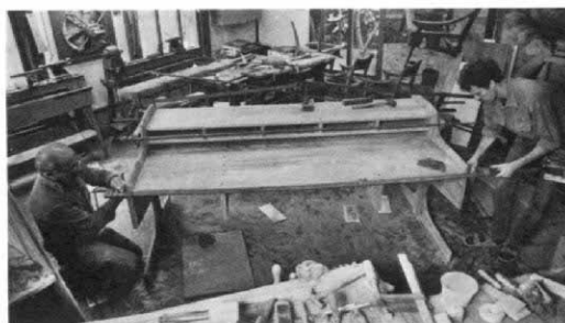
Assistant Jerry Marcotte helps position an 8-ft. bar clamp on a brown oak desk.
