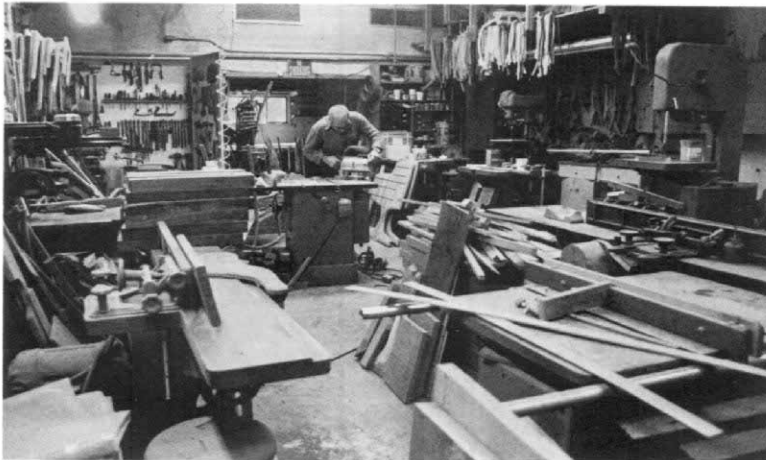
The 1,000-sq. ft. machine room is the largest of the three rooms that make up Maloof's shop. He's got two table saws, an 18-in. planer, two jointers (16 in. and 8 in.), a 20-in. and a 14-in. bandsaw, a 1-in. shaper, two cut-off saws, a hollow-chisel mortiser, a drill press, a horizontal-boring machine, two disc sanders and three lathes. Maloof's tool cabinet, right, is well stocked with routers, rasps and files.
