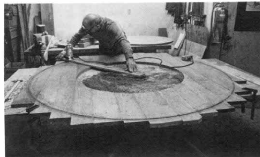
Router on trammel rounds a 6-ft. pedestal table. Inner circle will contain a lazy susan.
