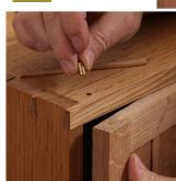
Use a dab of five-minute epoxy to ensure the parts don't shift. Insert the cup in the door with its slot parallel to the door front. Then insert the catch through the top of the case. The hole will be plugged with a dowel, but leave it long and use it to adjust the depth of the catch. The door should close with a nice click. Trim the dowel flush or round it and leave it slightly proud of the surface.
